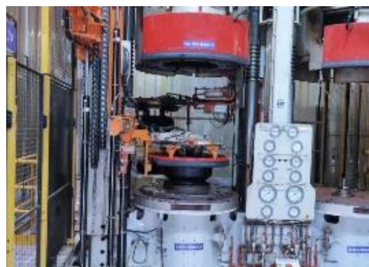
Transferring of Green Tyre from VCL Arm to Curing press
