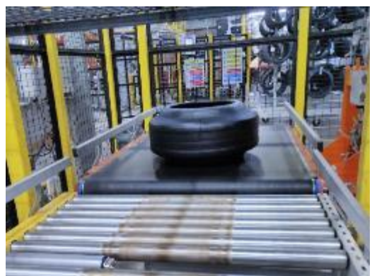
Transferring of Green Tyre from Conveyor to ASRS
