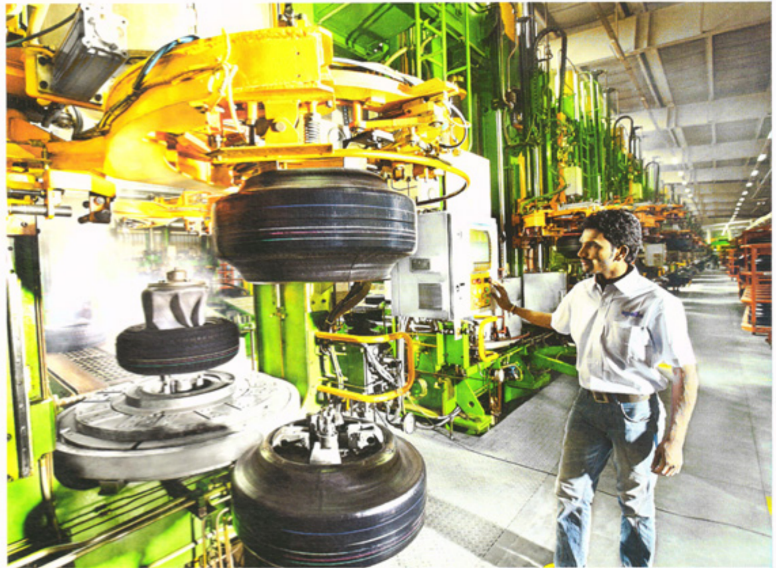
Tyre curing underway at the Chennai plant, which has state-of-the-art facilities.
